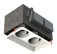
6. Compress springs on updated trim assembly and insert into slots in housing. Push up until secured into place.
